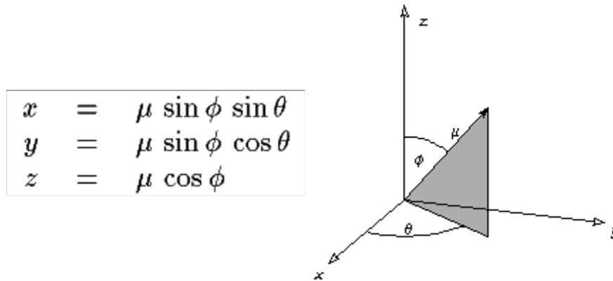
Figure 2-1. Spherical Coordinates
