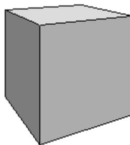
Figure 1-2. perspective projection (2 vanishing points)
